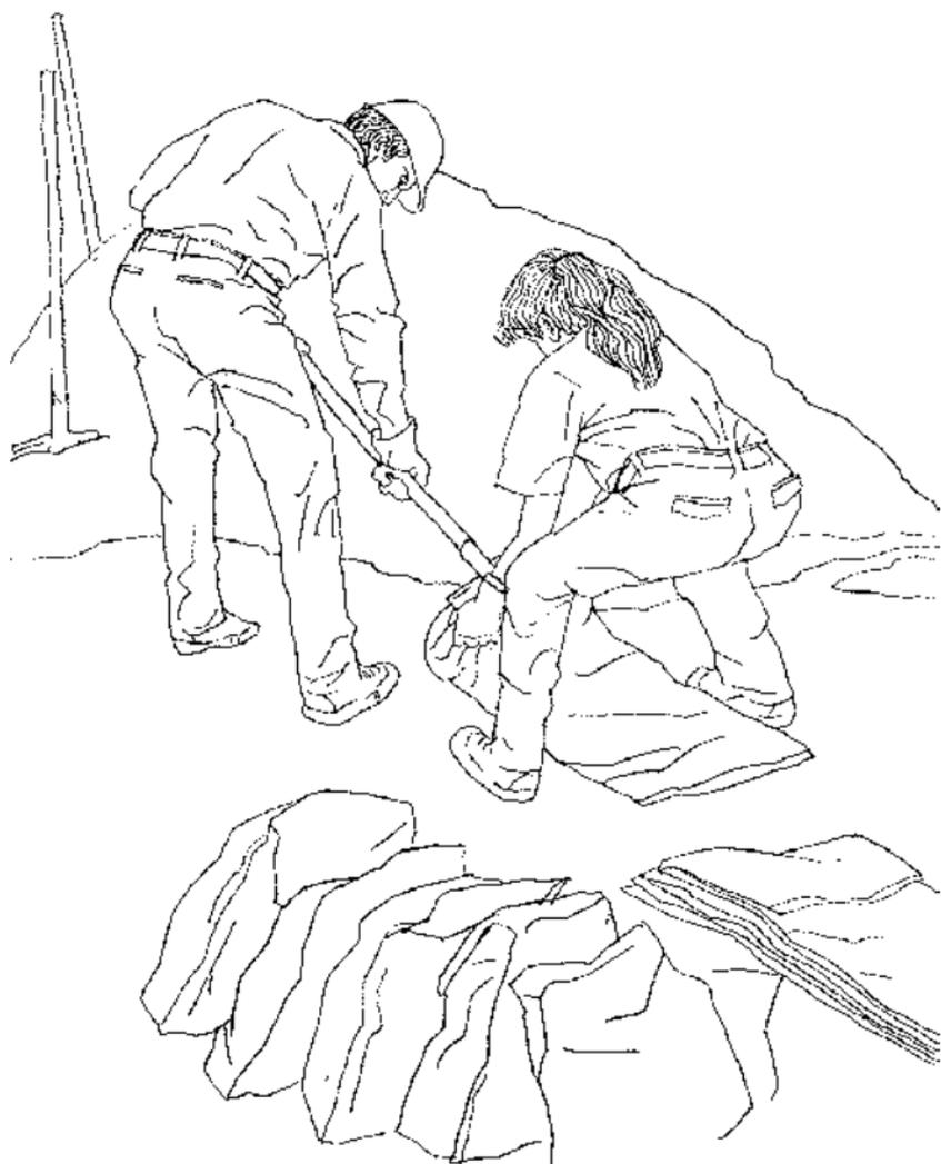
Figure 1: Proper sandbag filling
