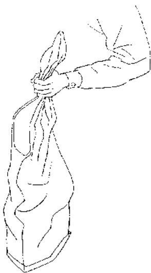
Figure 12A: Sandbag filled \frac{1}{4} to \frac{1}{3} full
